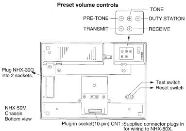
10 connector lead wires: connect to NHX-80X with 10 (5P) cable using wire nuts.
