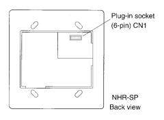
Plug in the supplied connector for wiring to NHX-80X.
