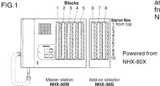
As shown in Fig. 1, the vertical rows of Call buttons are assigned sub station  $\#1 \sim 10$  (from top) of Trunks 1 - 5 from the left on NHX-50M.
