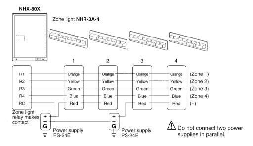
Wiring on NHX-80X CCU \* Use UL Listed cable for all wiring.
