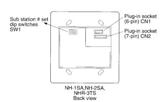
Plug in the supplied connector for wiring to Sub Trunk line.
