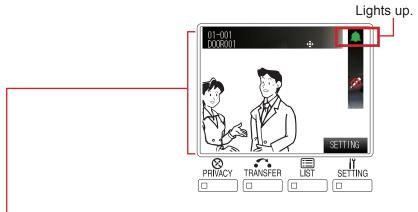
The station no., station name and video image at the calling station (following the symbol image) are displayed. (When called from a remote site, the site no., site name and video image at the calling station (following the symbol image) are displayed. The station name will not be displayed.)
